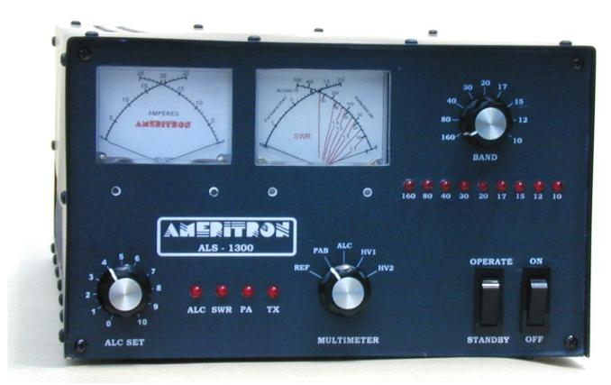
The Ameritron ALS-1300 is a 160 through 15-meter 1200-watt output solid-state amplifier. An optional user-installed MOD-10MK filter assembly extends operation to 12- and 10-meters. The ALS-1300 uses eight 50-volt conservatively rated linear RF MOSFETS. These 50-volt linear FET's produce an exceptionally clean signal compared to other solid-state amplifiers. Fan speed is regulated by temperature sensors assuring conservative cooling with minimum noise.
