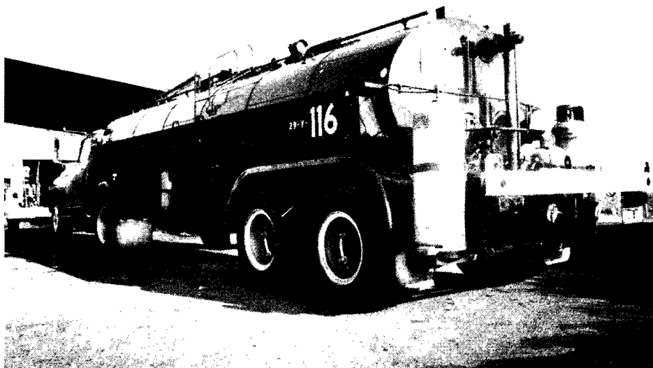
Above: One of the Board's 9000 litre bitumen road tankers after conversion to hydraulic pumping and LP gas heating systems
