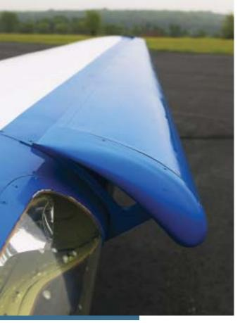
The wings-in-water design (above) increases lateral stability on the water and maximizes the benefits of ground effect during takeoff and landing. An 11-foot-long fixed slat (left) on each wing reduces stall speed and compensates for the absence of wing flaps.
