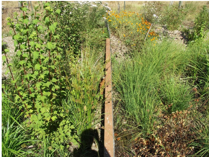
Figure 22. Biofiltration Cells at Study Site After 3 Years with a Complement of Native Plants. Treatment (mycoremediation) cell is on the left, control (bioretention only) cell on the right
