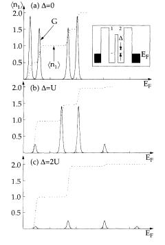
FIG. 3. Conductance spectra G (solid line) for different degrees of detuning  $\Delta$  of the second quantum dot against the first quantum dot (inset). (a)-(c) show G on the same scale for  $\Delta=0$ ,  $\Delta=U$ , and  $\Delta=2U$  in arbitrary units. Dashed line shows the average number of electrons in the first quantum dot ( $\langle n_1 \rangle$ ).
