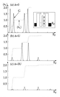
FIG. 3. Conductance spectra G (solid line) for different degrees of detuning  $\Delta$  of the second quantum dot against the first quantum dot (inset). (a)-(c) show G on the same scale for  $\Delta=0$ ,  $\Delta=U$ , and  $\Delta=2U$  in arbitrary units. Dashed line shows the average number of electrons in the first quantum dot ( $\langle n_1 \rangle$ ).
