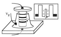
FIG. 1. Proposed experimental setup for a sidewall-gated small-cross-section vertical triple barrier structure. Inset shows the simplified conduction band in the central region in the growth direction. Fermi energy and lateral confinement can be changed with the gate voltage  $V_g$ .
