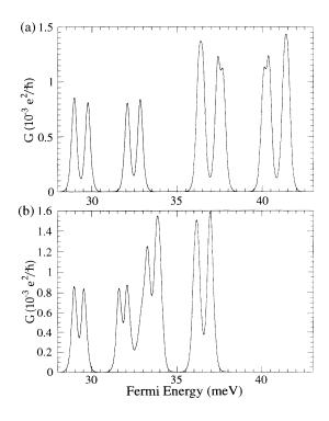
FIG. 8. Conductance spectrum calculated with  $\epsilon_0 = 30$  meV, t=1 meV,  $k_BT=0.1$  meV, and the interaction energies calculated with the screened Coulomb potential [Fig. 6(c)] for two different quantum dot sizes (a)  $d_x = d_y = 550$  Å and (b)  $d_x = d_y = 750$  Å.
