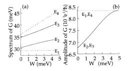
FIG. 5. (a) Conductance peak spectrum as a function of interdot charging W. First peak is unchanged, fourth peak changes linearly with interdot charging. (b) Amplitudes of conductance peaks. Dashed line corresponds to peaks 1 and 4 in (a). Peaks 2 and 3 (solid line) increase until all four peaks have the same amplitude at W=U where interdot and intradot charging energies are the same.
