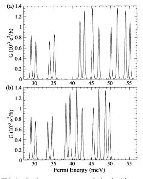
FIG. 7. Conductance spectrum calculated with  $\epsilon_0 = 30$  meV, t=1 meV,  $k_BT=0.1$  meV, and the interaction energies calculated with the saturated Coulomb potential [Fig. 6(b)] for two different quantum dot sizes (a)  $d_x = d_y = 550$  Å and (b)  $d_x = d_y = 750$  Å.
