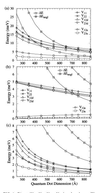
FIG. 6. Direct  $(V_{11}, V_{22}, V_{12d}, V_{23d})$  and exchange  $(V_{12e}, V_{23e})$  Coulomb integrals and single-particle excitation energies  $\Delta E = E_2 - E_1$  and  $\Delta E_{negl}$  as a function of lateral confinement  $d_x = d_y$  for (a) unscreened Coulomb potential, (b) saturated Coulomb potential ( $\alpha = 200$  Å), and (c) screened Coulomb potential ( $\beta = 50$  Å).
