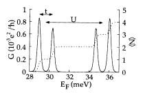
FIG. 2. Conductance G (solid line) calculated for a system of coupled, symmetric quantum dots as a function of Fermi energy  $E_F$ . Conductance peaks are grouped by charging energy U and coupling energy t. Transitions in the total number of electrons N (dashed line) in the quantum dot coincide with the conductance peaks.
