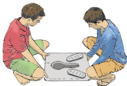
Figure 18. Lifting a sanplat
