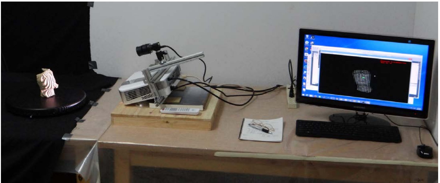
Figure 1. The custom-made, structured light set-up in the workroom of the Larnaka District Museum, Cyprus. The object is placed on a turn-table while the projector emits patterns of light while scanning. This is repeated every 45 degrees and on the top and bottom of the object. The ten scans are merged in the post-processing phases using custom software developed by the University of Kentucky's Center for Visualization and Virtual Environments.
