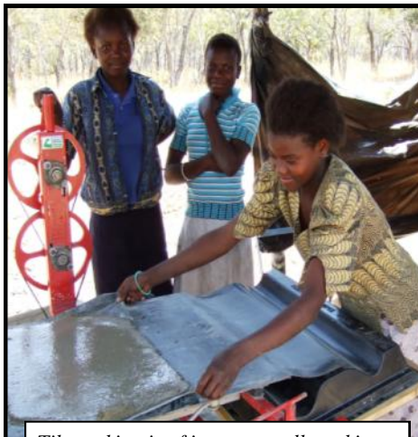
Tile-making is of interest to all: making a Super Roman tile for a school in Fiwila
