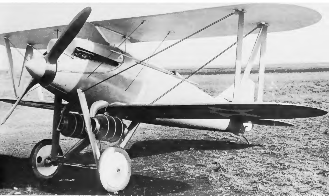
FIGURE 30.—Navy Curtiss Racer CR-1, powered by Curtiss CD-12 engine, 400 hp. This plane, piloted by Bert Acosta, won the Pulitzer trophy at Omaha, Nebraska, on 3 November 1921. (Smithsonian photo A-4624B.)
