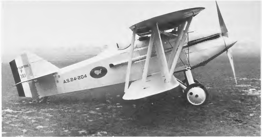
FIGURE 35. —Curtiss Pursuit PW-8, 1924. This plane, powered by a Curtiss D-12 engine and piloted by Lieutenant R. L. Maughan, flew the “Dawn to Dusk Flight” of 2,700 miles from New York to San Francisco in 21 hours and 48 minutes on 23 June 1924. (Smithsonian photo A-4655G.)
