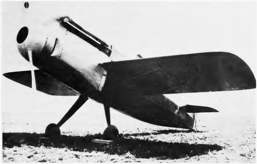
FIGURE 43.—Steve Wittman's Bonzo racer, powered by a Curtiss D-12. (Photo courtesy of Experimental Aircraft Association. Smithsonian photo A-5083A.)
