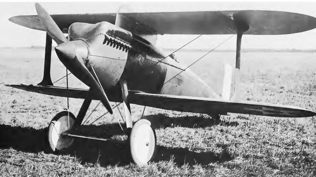
FIGURE 31.—Curtiss R-6 Army racer powered by Curtiss D-12 engine, 450 hp, 1922. (Smithsonian photo A-4624E.)
