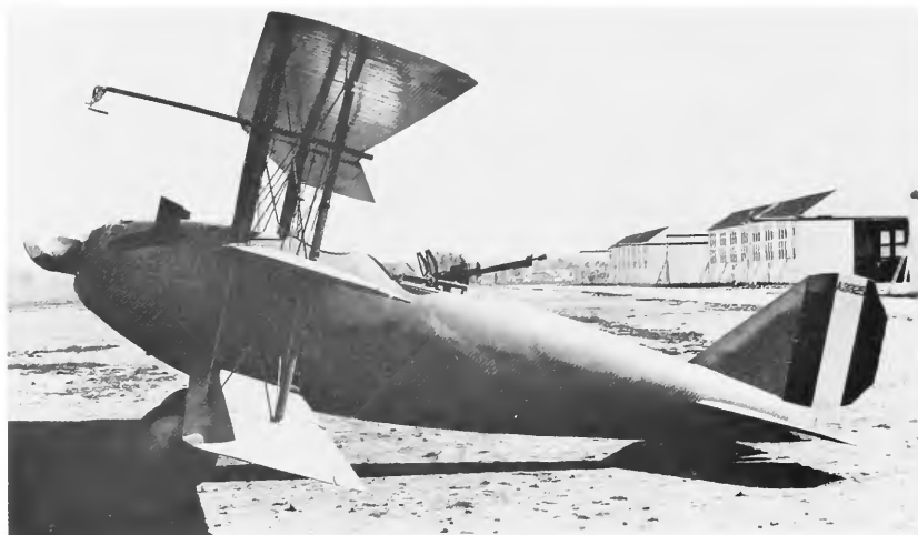
FIGURE 13.—Curtiss-Kirkham 18-T Wasp triplane, about 1919, with Curtiss K-12 engine, 1918. (Smithsonian photo A-4597.)
