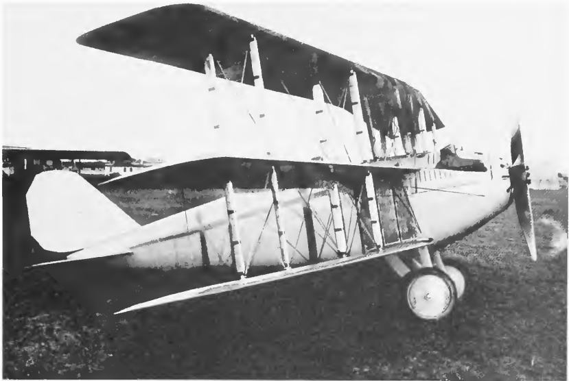
FIGURE 21.—Curtiss 18-T Wasp with Curtiss K-12 engine, destined for Bolivian air force, October 1919. (Smithsonian photo A-4602G.)
