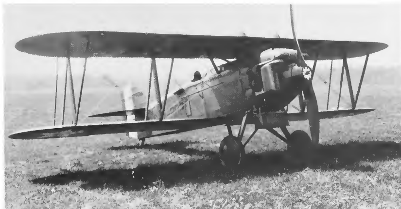
FIGURE 39.—Curtiss PW-8 pursuit plane of 1924, powered by a turbosupercharged Curtiss D-12. (Smithsonian photo A-4667B.)
