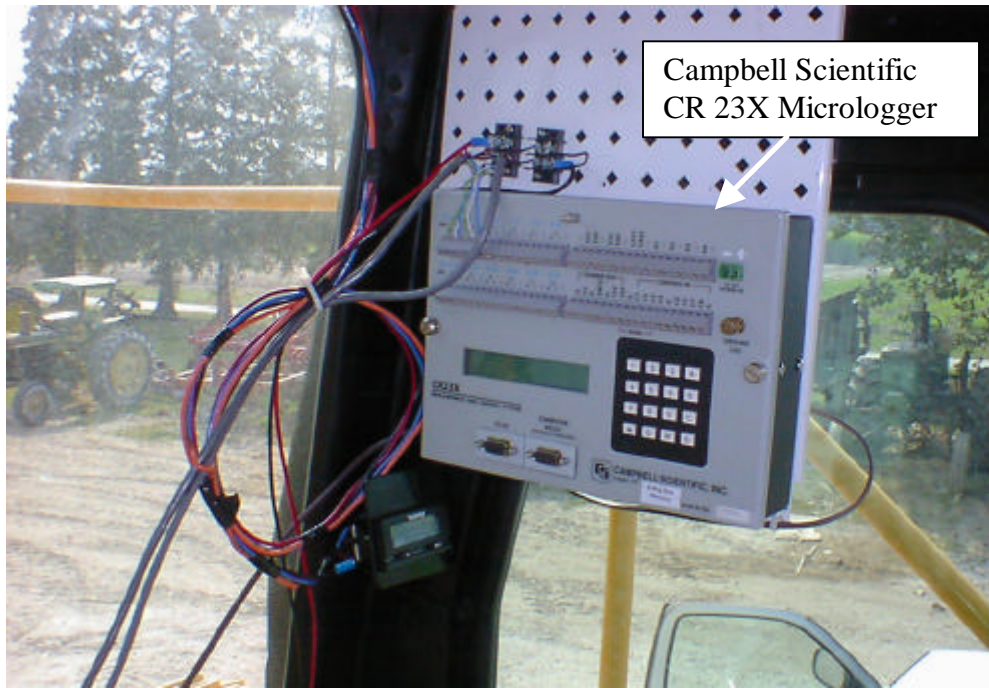
Figure E3. Data-logger inside the Harvester's Cab
