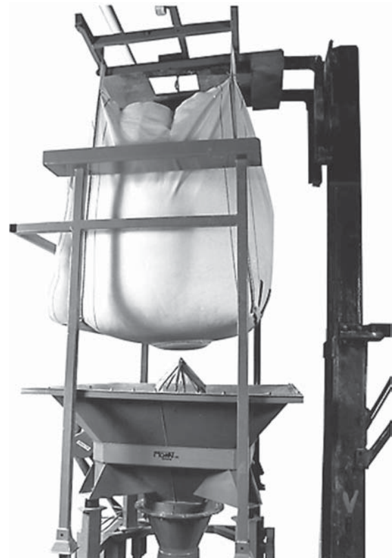
Figure 1. The most popular style of bulk bag: dispensed from the bottom. (Photo courtesy of Control and Metering Ltd.)
