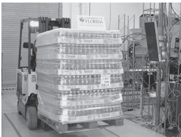
Figure 14. A pallet passes through an RFID portal in the packaging laboratory at the University of Florida. (Photo by Bruce Welt, University of Florida.)
