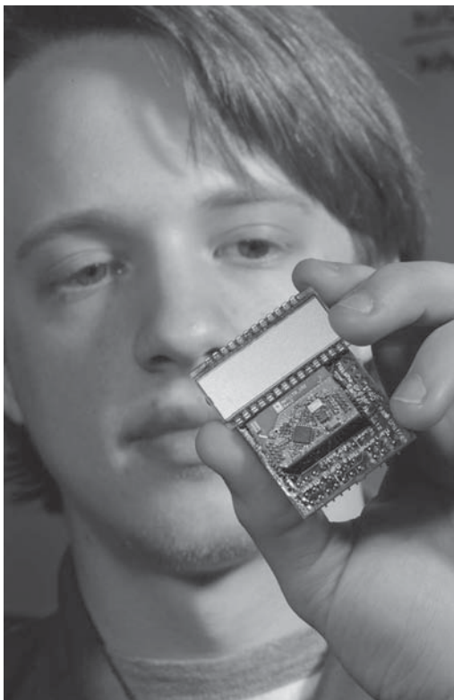
Figure 3. Active RFID freshness monitoring tag developed at the University of Florida.
