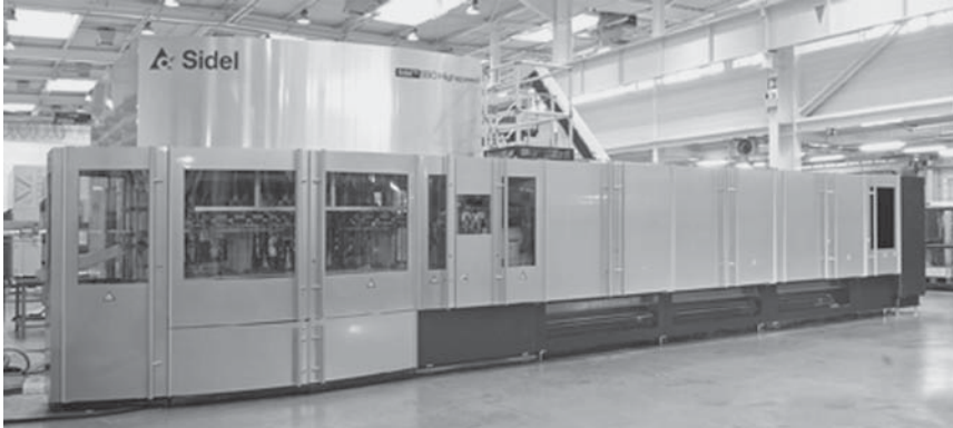
Figure 13. A horizontal rotary two-step blow-molding machine with preform oven. This is a high-output machine featuring 34 blowing stations capable of manufacturing over 61,000, 0.7-L carbonated soft drink PET bottles per hour. (Courtesy of Group Sidel.)
