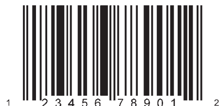
Figure 6. UPC barcode example for (123456789012).
