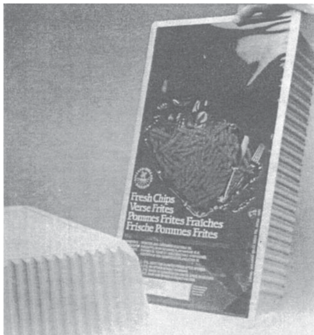
Figure 2. Modified atmosphere package for perishable foods. Fresh (unfrozen), precooked French fries (10 kg) packed in N_2 atmosphere. Positive (male) formed PVC/PE bottom, polyester/PE cover. Print registration of flexible upper web by means of stretching with a brake.
