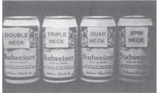
Figure 4. Double-, triple-, quadruple-, and spin-neck can.
