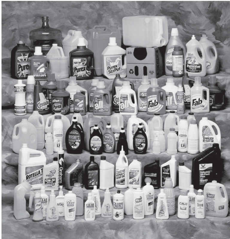
Figure 1. An array of extrusion blow-molded bottles. (Courtesy of Graham Engineering Corporation.)
