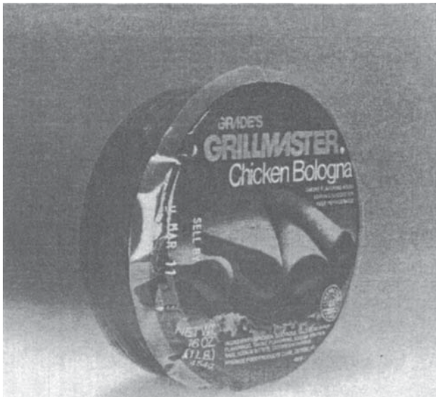
Figure 6. Sliced luncheon-meat package. Nylon-ionomer flexible forming web, OPET/ionomer top web. Circle cutting by means of flying knife. Print registration by means of stretching film with a brake.
