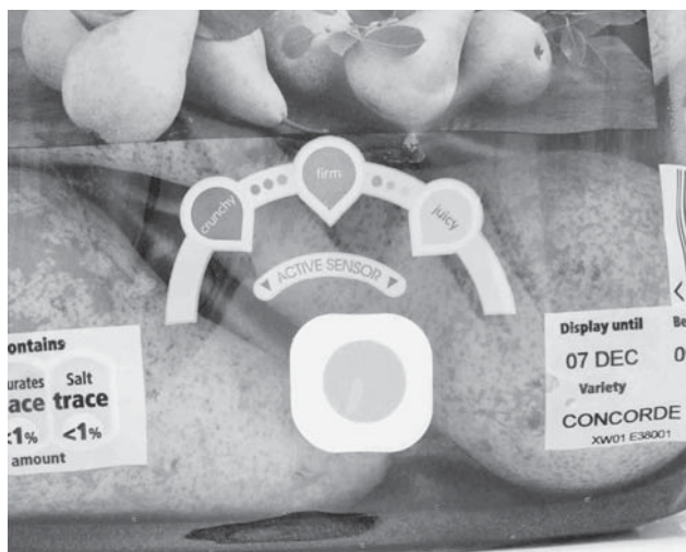
Figure 10. A pack of four Concorde pears with active ripeness indicator. The label inside the pack changes color from dark red to yellow as the pears ripen.
