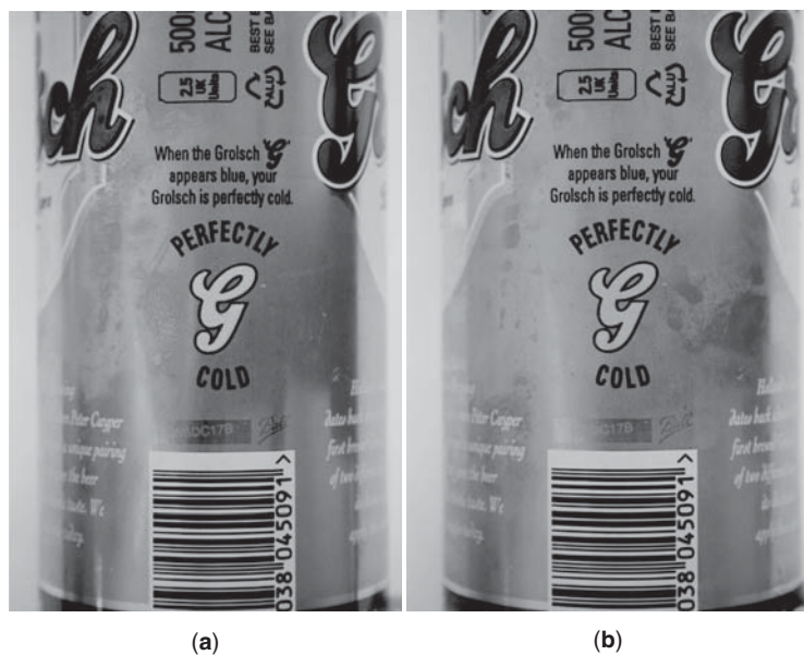
Figure 1. Photographs of a can of Grolsch™ beer (a) before and (b) after correct chilling, the ink in the label becomes lighter.
