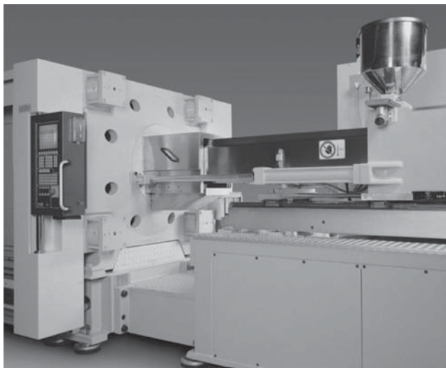
Figure 10. The injection unit displayed here shows a stainless steel purge guard over the heated barrel and hydraulic carriage cylinders (both sides). (Photo courtesy of Negri Bossi.)
