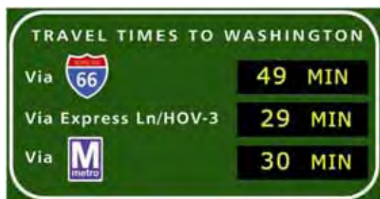
Figure 3.41 Multimodal Travel Times on Dynamic Message Signs
