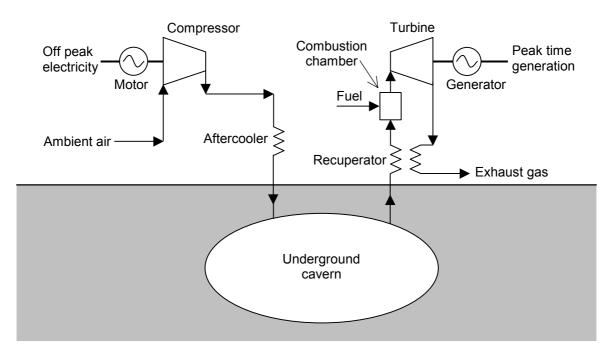
Figure 2.1 Schematic of a Compressed Air Energy Storage System
