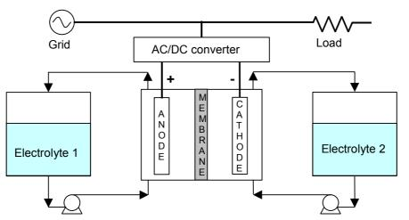
Figure 4.1 Schematic of a Redox Flow Cell Energy Storage System
