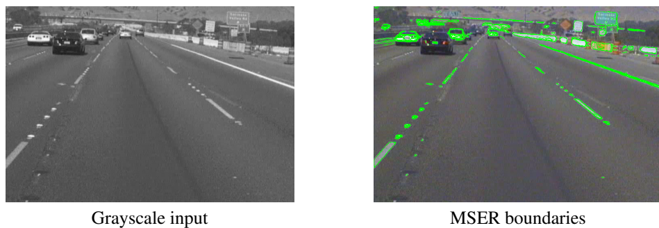
Figure 6: MSERs can be used for traffic lane and traffic sign detection.
