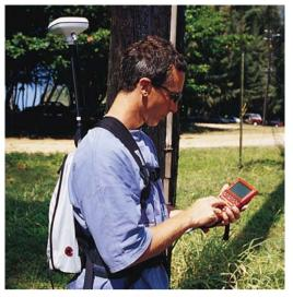
Fig 1.20 GPS surveying equipment used to produce the three dimensional topographical models of selected hillforts. a) Trimble Navigation 4600LS post-processing GPS equipment b) Leica Geosystems System 530 real-time kinematic equipment (from EH, Centre for Archaeology and courtesy of Leica Geosystems Ltd).
