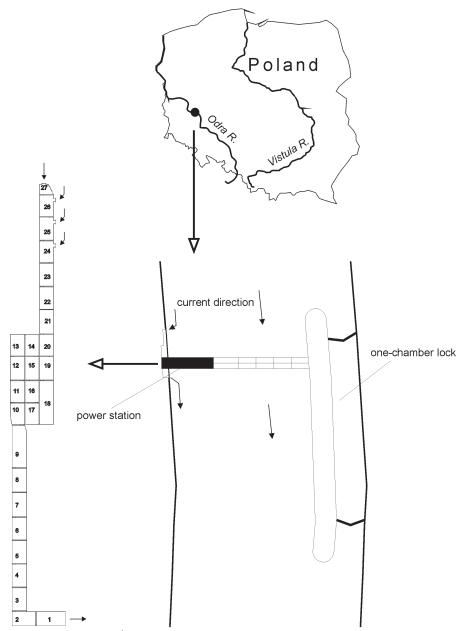
Fig. 1. Location of the dam "Wały Śląskie" and the scheme of the fish-pass. Small arrows indicate the water flow direction.
