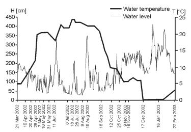
Fig. 2. Water temperature and water level values obtained from the permanent measuring point near Wały Śląskie in the study period.
