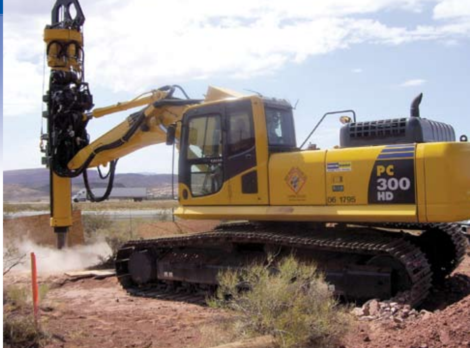
A Most Wanted Drilling operator works a Komatsu PC300HD-8 excavator equipped with a DH60-60 LoDril attachment.
