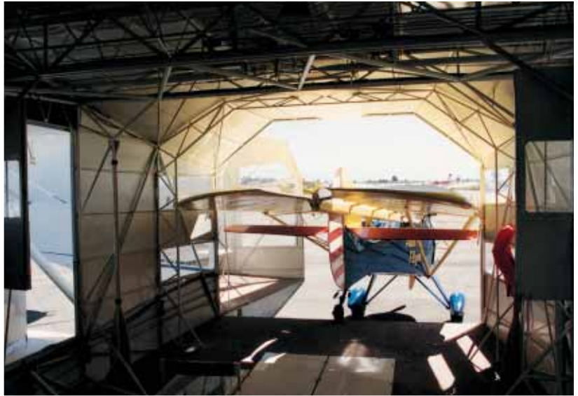
The Explorer's fuselage opens for cargo loading. Here, an Avid Flyer with wings folded makes its way inside. A Robinson R-22 helicopter, minus the rotor blades, can fit, too.
