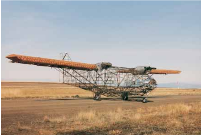
The under-construction Twin Explorer awaits its covering job. The massive machine weighed in at 5000 pounds empty.
