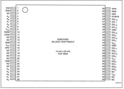
Figure 2-16. 28F016XD 56-Lead TSOP Type I Pinout Configuration
