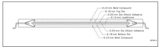
Figure 5-4. DDTSOP Cross Section
