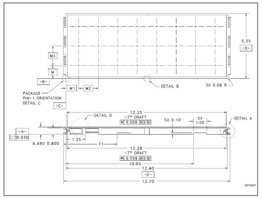
Figure 7-1. SOP Thick Tray Diagram
