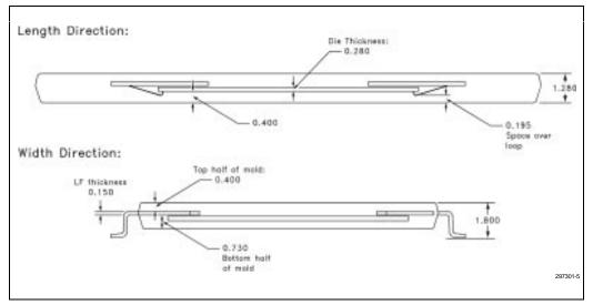
Figure 5-5. 56-L SSOP Cross Section
