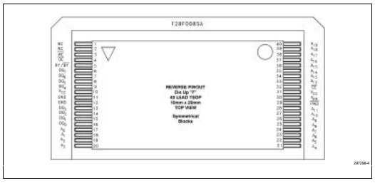
Figure 2-4. 40-Lead TSOP Package Pinout for 28F008SA—Reverse Pinout
