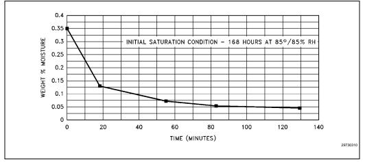
Figure 7-17. TSOP Desorption at 125 °C
