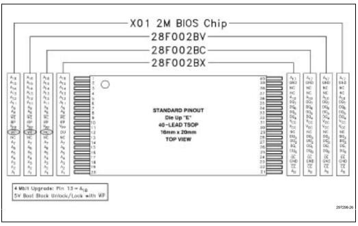
Figure 2-7. The 40-Lead TSOP Pinout for X01 2M BIOS, 28F002BV, 28F002BC, and 28F002BX
