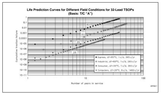
Figure 6-1. 32-Lead TSOP Life Prediction Curves
