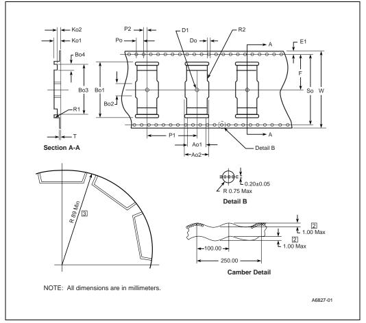
Figure 7-5. TSOP Tape and Reel Carrier Tape Diagram
