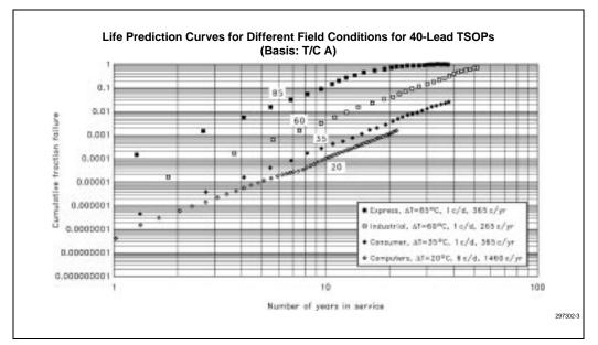
Figure 6-3. 40-Lead TSOP Life Prediction Curves
