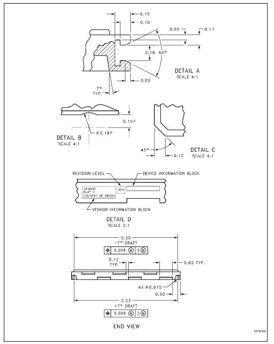
Figure 7-2. SOP Thick Tray Diagram (Detailed View)
