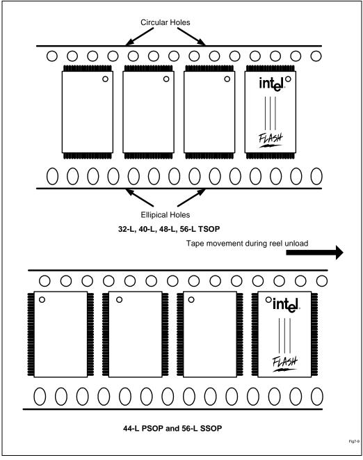
Figure 7-8. SOP Tape and Reel Orientation
