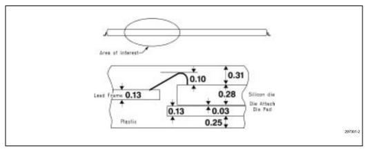
Figure 5-2. Typical TSOP Cross Section
