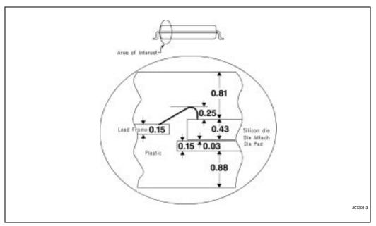
Figure 5-3. PSOP Cross Section
