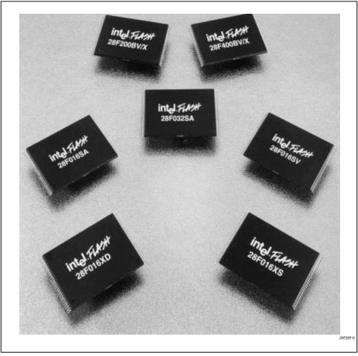
Figure 1-5. 56-Lead TSOP Package
