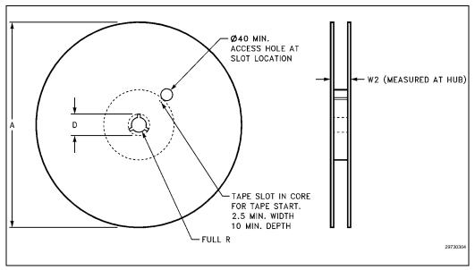
Figure 7-7. SOP Carrier Tape and Reel Dimensions
