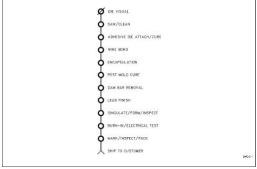
Figure 5-1. SOP Assembly Flow Chart
