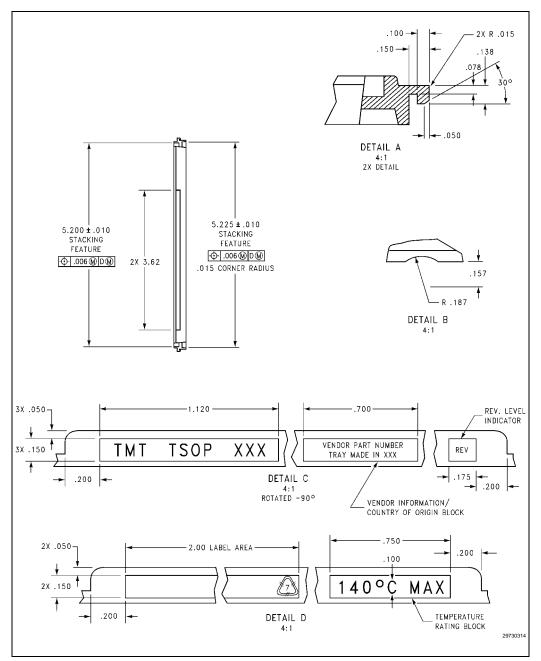
Figure 7-4. SOP Thin Tray Diagram (Detailed View)
