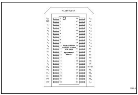
Figure 2-11. 44-Lead PSOP Package Pinout for 28F008SA
