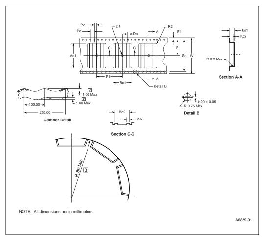
Figure 7-6. 44 mm, 44-Lead PSOP/56-Lead SSOP Tape and Reel Carrier Tape Diagram
