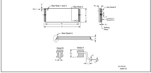
Figure 3-1. 32-Lead TSOP Package Drawing and Specifications
