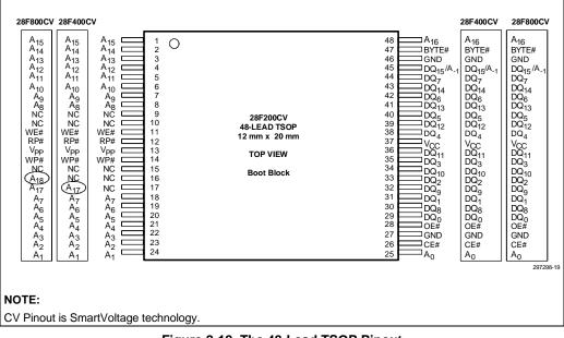
Figure 2-12. The 48-Lead TSOP Pinout for 28F200CV, 28F400CV and 28F800CV
