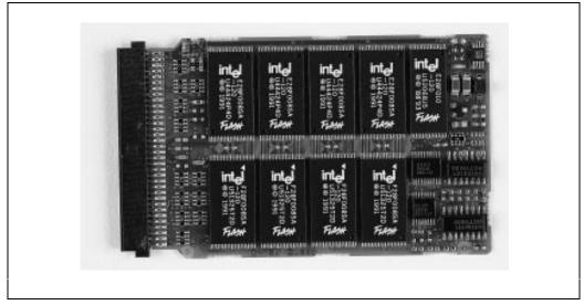
Figure 2-19. TSOP Is Ideal for Memory Card Applications
