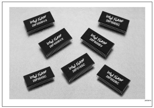
Figure 1-6. 44-Lead PSOP Package
