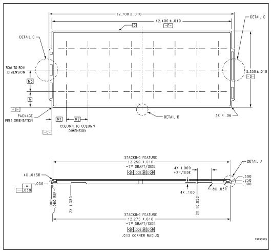
Figure 7-3. SOP Thin Tray Diagram
