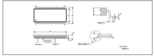
Figure 3-5. 44-Lead PSOP Package Drawing and Specifications
