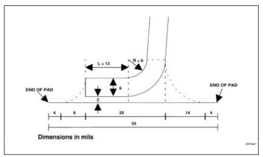
Figure 8-1. TSOP Lead Placement Close-Up View
