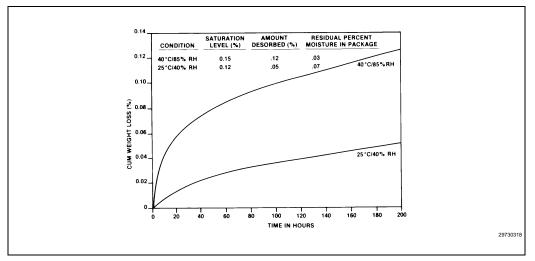
Figure 7-10. Saturated Component Weight Loss at Low Temperature
