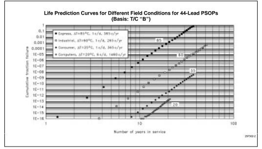
Figure 6-2. 44-Lead PSOP Life Prediction Curves
