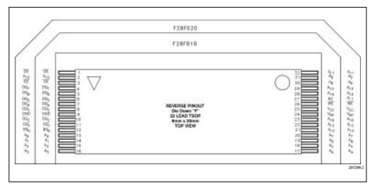
Figure 2-2. 32-Lead TSOP Package Pinout for 28F001BX, 28F010 and 28F020—Reverse Pinout
