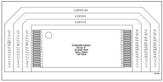
Figure 2-1. 32-Lead TSOP Package Pinout for 28F001BX, 28F010 and 28F020—Standard Pinout
