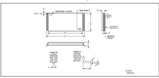
Intel's 40-lead TSOP meets the EIAJ and JEDEC registered standard.
