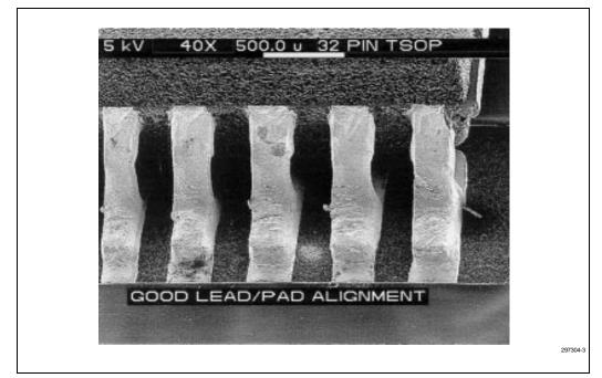
Figure 8-3. Example of Good Placement
