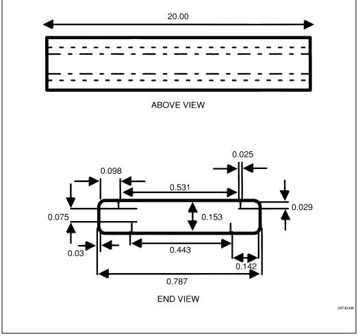
Figure 7-9. 44-Lead PSOP Shipping Tube
