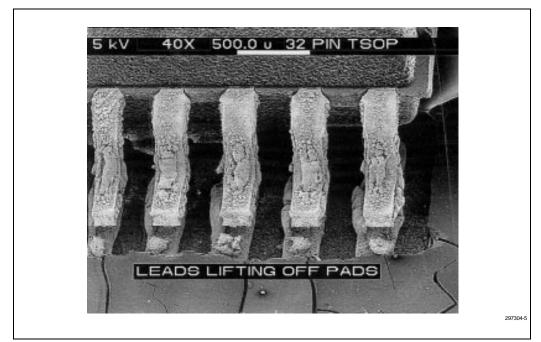
Figure 8-5. Example of Lifting
