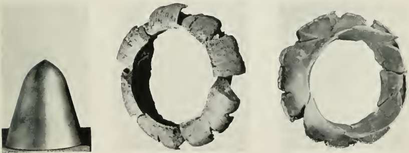
Diagram showing Cap Action on Armour-Piercing Projectiles.
