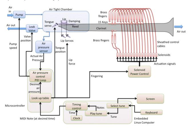
Figure 2. A schematic of the clarinettist showing the mechanisms and controllers. Not to scale.
