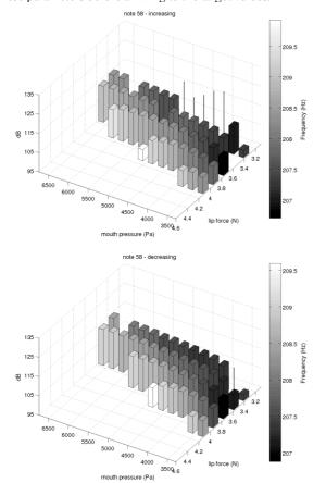
**Figure 4:** Plots of playing frequency as a function of air pressure and lip force f(P,F) for the note (written A#3). In this run, F was held constant while P was increased (top) or decreased (bottom). Narrow columns are 'wrong' notes produced with this fingering, usually squeaks.
