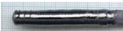
Figure 1. Photograph of an artificially grown single crystal of \text{CoNb}_2\text{O}_6 . The experiment involved a 2-centimeter-long piece of this crystal, weighing about 8 grams. (Image courtesy of Radu Coldea.)
