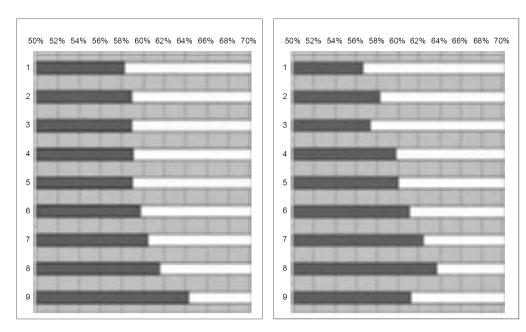
Figure 15. Percent composition (RDX = blue; DNAN = cream) of ARX-4027m1 (left) and m2 (right) along a 25.4 x 200 mm cylinder- using 20 mm long samples. The y axis represents 9 sectioned charges (20 mm length), with 9 at the bottom.
