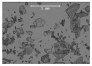
Figure 10. Micrograph of RDX plates recrystallised from DNAN. Typical crystals were 0.01 - 0.02 mm thick.
