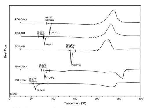
Figure 3. DSC for relevant 50:50 (wt/wt) mixtures
