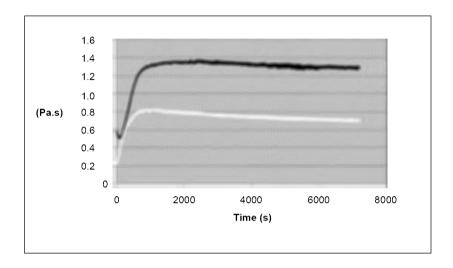
Figure 14. Viscosity profile for ARX-4027 (yellow) and Composition B (blue)
