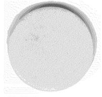
Figure 11. ARX-4027 poured into and cooled in a steel pan (left), and a 1-inch disc cut from a stick of ARX 4027 (right).
