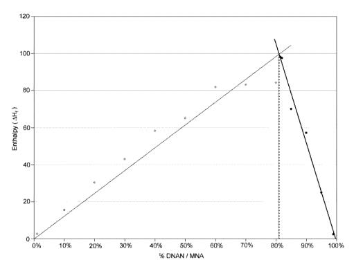
Figure 5. Plot of Enthalpy of Fusion ( $\Delta H_f$ ) vs %DNAN (by wt) in a mixture of DNAN/MNA showing the  $\Delta H_f$  (eutectic) maxima at 82 (±1)% DNAN.<sup>10</sup>
