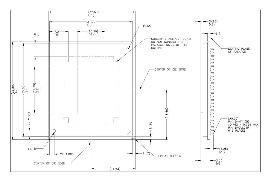
Figure 1a: 615-pin Micro-PGA package top and side view (see Figure 1b for package dimension).
