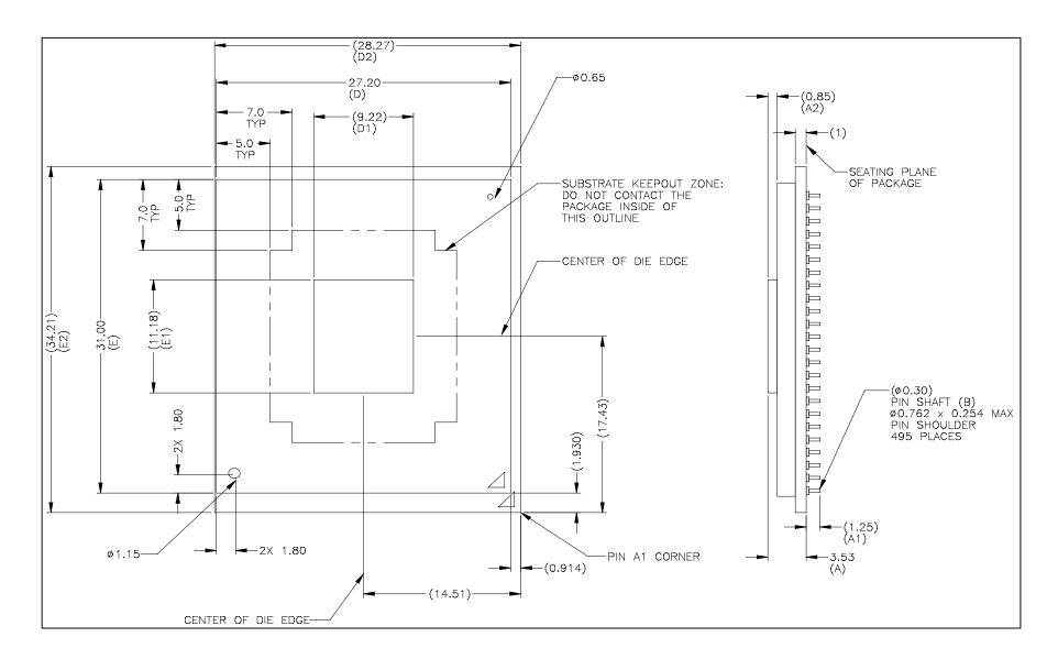
Figure 2a: 495-pin Micro-PGA package top and side view (see Figure 2b for package dimension).
