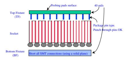
Figure 10: Cross-sectional view of the top and bottom L fixtures
