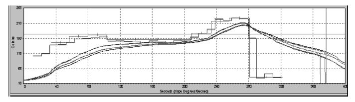
Figure 8: Typical Reflow Profile for 63Sn/37Pb solder
