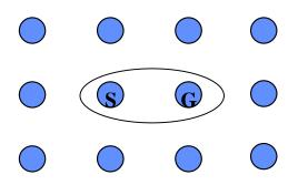
Figure 12: Pin layout for capacitance meaurements
