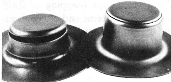
Figure 14-2 Drawing failures by necking at bottom of cup wall. With very low friction, the failure site tends to move onto the punch radius as shown at the right. From D. J. Meuleman, Ph.D. thesis, Univ. of Michigan (1980).
