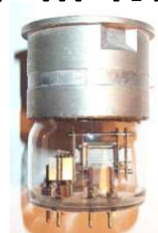
Telefunken LG2 Dual Diode Würzburg RX Mixer (NF 16 dB)
