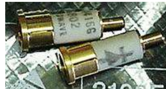
1N416 Si Mixer Diodes: used in US and British radar receivers (NF 6 – 7 dB)
