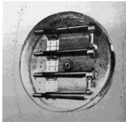
4-element polyrod antenna, downward-looking & rotating at 400 rpm.
