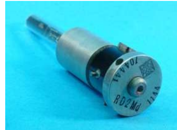
RD 2 Md split-anode magnetron: (3 GHz, 0.4W CW) used as RX LO in all Berlin 9 cm radars
