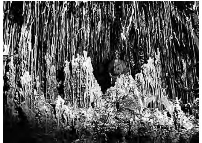
Figure 4. Halite speleothems formed from brines seeping into coal workings from the Permian evaporites, Westoe Colliery, South Shields (Photo: A Doyle).
