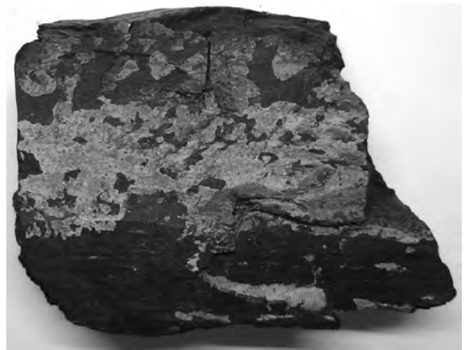
Figure 2. Sample of Durham Main coal seam with abundant ankerite mineralisation on cleat surface.
