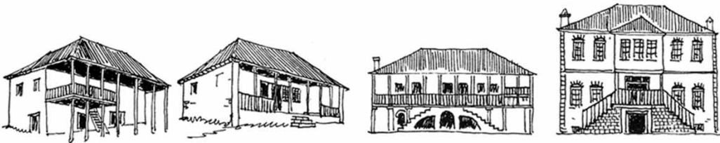
Figure 2. Non-defensible Ottoman-era house typologies in Albania. From the left: vatër zjarri type, hajati type, çardak type, and qoshkë type. Illustrations courtesy of Emin Riza and Pirro Thomo.
