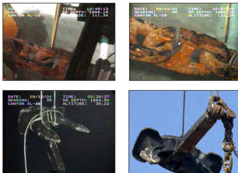
Figure 5-42. The Anchor Chains Were Cut and the Anchors Removed from the Hawse Pipes.
