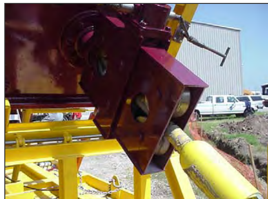
Figure 5-31. Nozzle Exiting Coiled-Tubing Drilling System.
