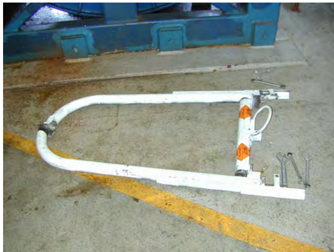
Figure 5-21. Shaped Explosive Charge Tool to Aid in Removal of the Center Mast.
