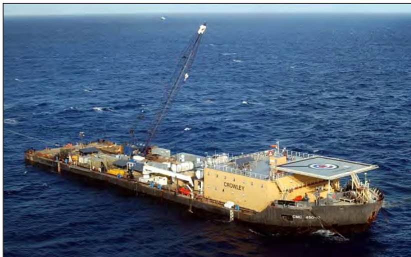
Figure 5-64: Crowley 450-10 with EHIME MARU Suspended Underneath Being Towed to the Deep-water Relocation Site.
