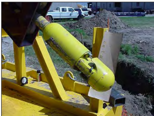
Figure 5-31. Nozzle Exiting Coiled-Tubing Drilling System.
