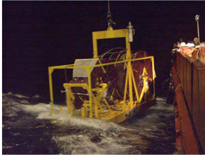
Figure 5-32. Launching Coiled-Tubing Drilling System.
