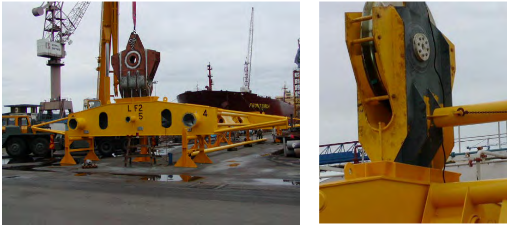
Figure 5-43. Lower Lifting Assembly During Fit Out with One Upper Sheave.
