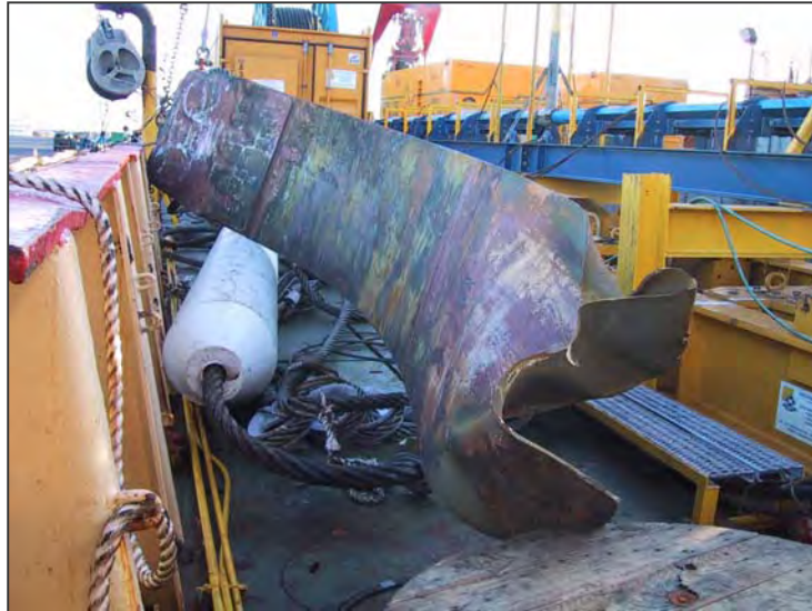
Figure 5-35. Broken Lifting Plate After Stern Lift.
