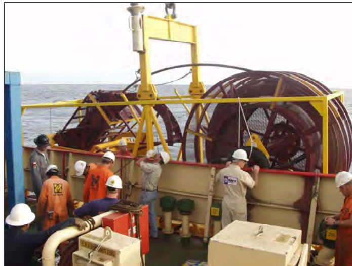
Figure 5-33. Coiled-Tubing Drilling System Being Deployed.
