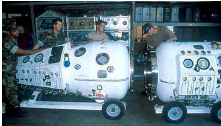
Figure 5-58. Transportable Recompression Chamber System (TRCS).
