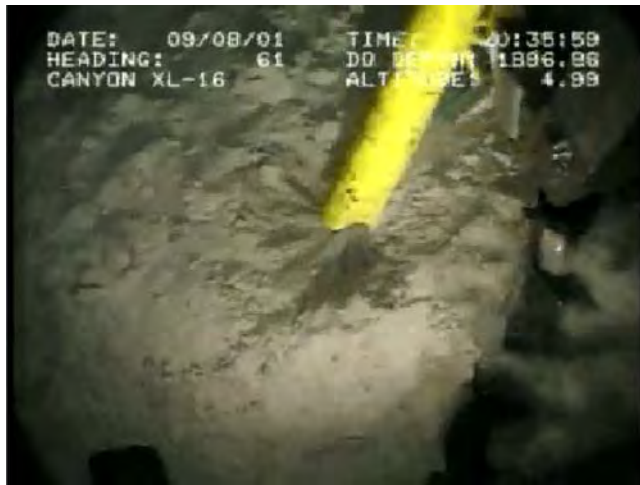
Figure 5-40. Suction Hose Removing Bow Sediment.
