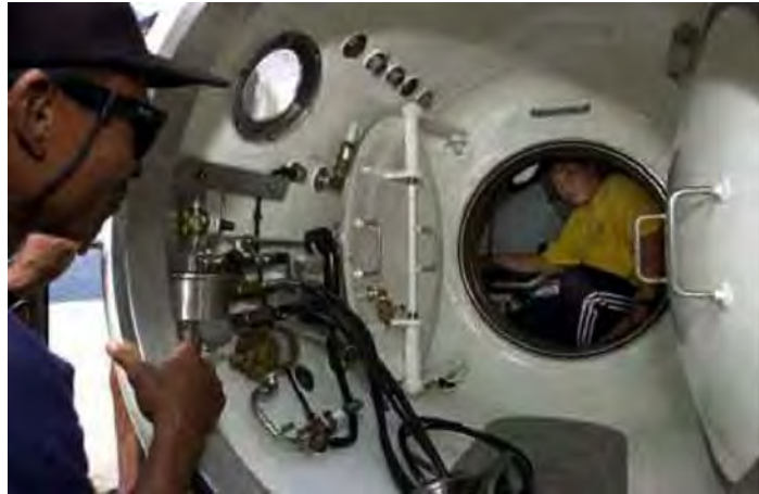
Figure 5-57. Transportable Recompression Chamber.
