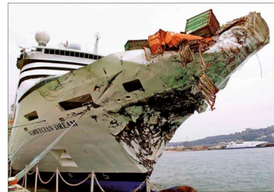
THE preoccupation of the watchkeeper with the ship's garbage return documentation contributed at least in part to the nearly calamitous collision between the cruiseship Norwegian Dream (above) and a containership in the North Sea. (Photo: Reuters)
