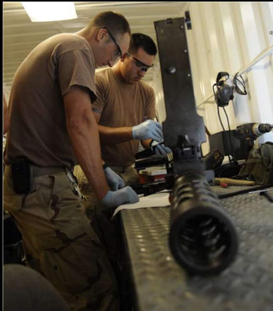
Coast Guard Maritime Enforcement Specialist's 2 nd Class Zachary Houghton and Micahel Maldonado clean a .50-caliber Browning machine gun.
