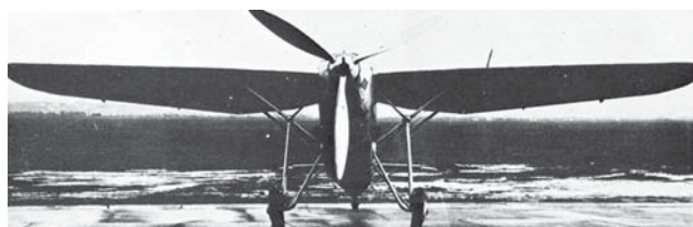
Ikarus IK-02, view from the front, center on the complicated structure of the landing gear and wing struts. Image created during testing in October in 1936. Airfield Zemun. Photo Dobnikar collection
