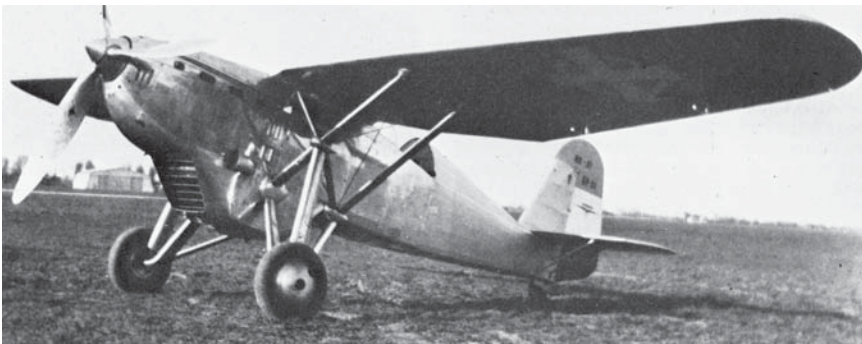
Ikarus IK-L1 with aerodynamic trim removed landing gear, April 1935, Zemun airfield
