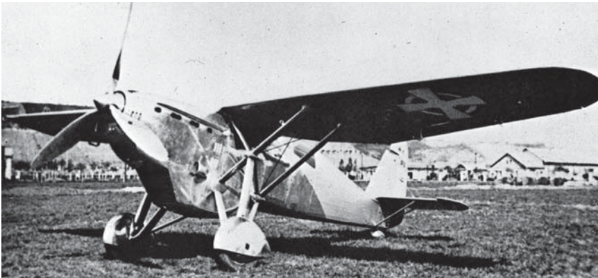
Ikarus IK-L1, with aerodynamic trim landing gear which have added some 8-10 km / h at a maximum speed of aircraft Ik-L1. Airfield Zemun, April 1935.
