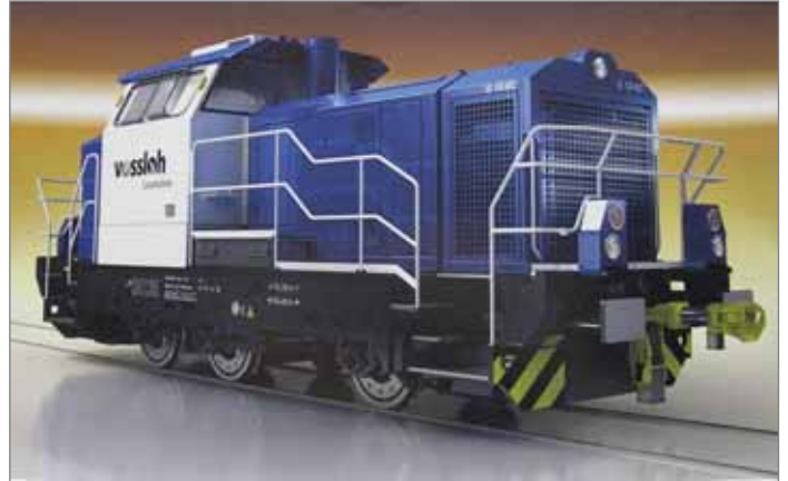
Vossloh G6 locomotive powered by QSK23
