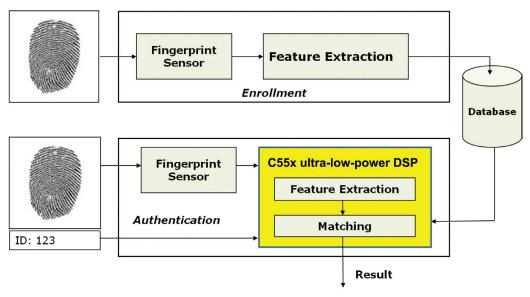
Figure 4: Block diagram of fingerprint process system.
