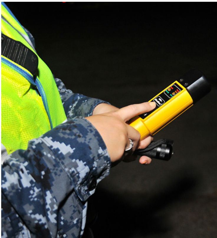
Master-at-Arms Seaman Apprentice Morgan Garnan with the U.S. Naval Station Guantanamo Bay Security Forces, explains the proper use of the "AlcoBlow" device used to determine if a person has any alcohol on their breath. The MA administers a sobriety test during a checkpoint Aug 15, at NAVSTA GTMO. (Photo by Sgt. 1st Class Marie Schult-Slosser)
