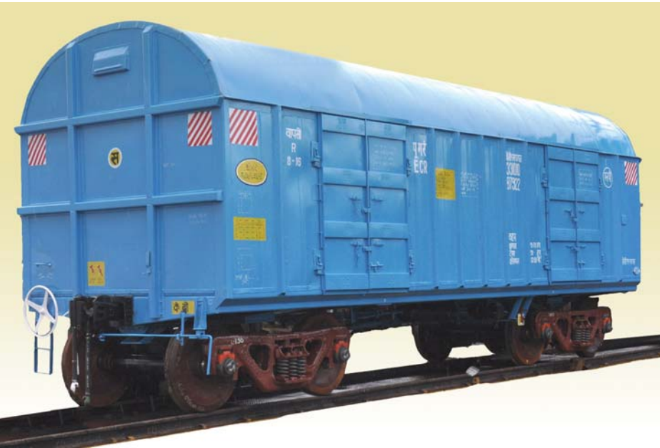
BCNHL stainless steel wagons provide 34% higher train throughput on IR.
