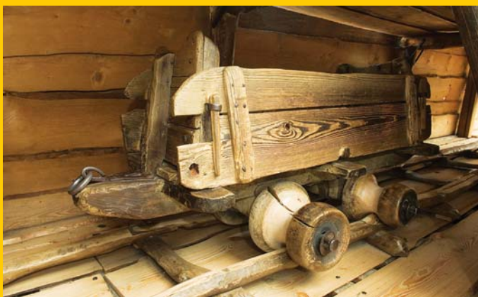
Wooden rails and mining cart from a Romanian silver mine, around 16th century (Photo courtesy : Clemens Kirchner, Deutsches Technikmuseum, Berlin)
