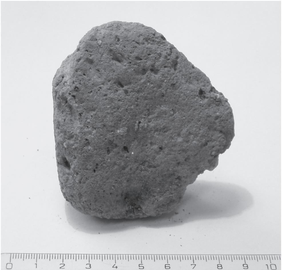
Fig. 11. A photo of the biggest piece of brick, found in a dug probe 80 cm deep. Notice the almost perfect roundness after merely 600 m transport.
