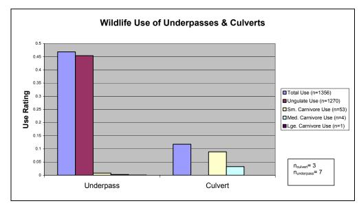
Fig. 2. The type and frequency of wildlife use compared between culverts and underpasses (Use Rating =  $(\Sigma \# of \text{ photographs})/(\Sigma \# of \text{ functional camera days})$ ). Ungulates used underpasses exclusively while small carnivores were more frequent users of culverts. Medium carnivores were found at both underpasses and culverts and one black bear was recorded using an underpass.Total use ratings included other wildlife and humans.
