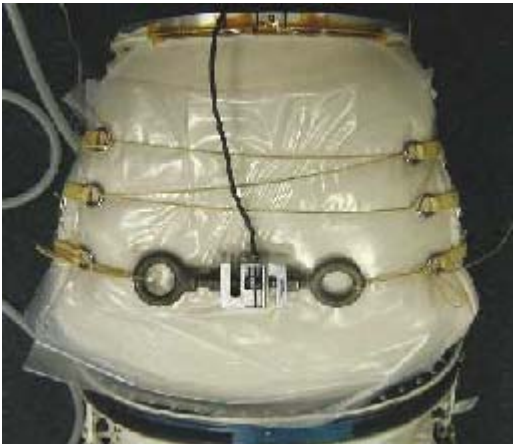
Figure 10: SUT at 4.3 psid with Load Cell
