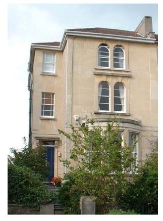
Figure 42: Typical semi-detached villa with side entrance and ground floor bay
