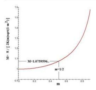
One can use this graph to check the iteration convergence. For example at m=0.8 one should expect M to be very near 1.31. Note that M approaches M=1 at m=0 and M $\rightarrow \infty$  at m=1.
