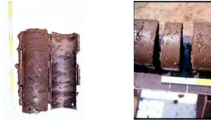
Figure 1 Soil sampler (left) and soil core (right) taken in the field trial.
