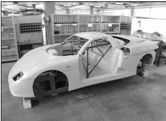
The body panel pieces are assembled and hand-fitted in a jig, then bonded together
