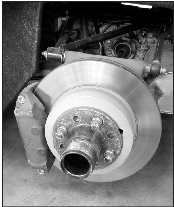
The front brakes feature massive calipers and fully vented and drilled rotors, while the rear brakes utilize smaller calipers and smaller vented rotors for lower unsprung weight
