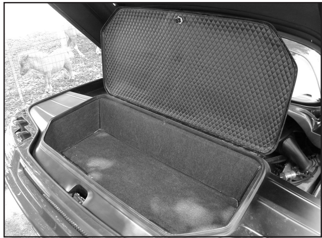
An insulated fiberglass box lies atop the gearbox to serve as a trunk, sized to hold two sets of golf clubs
