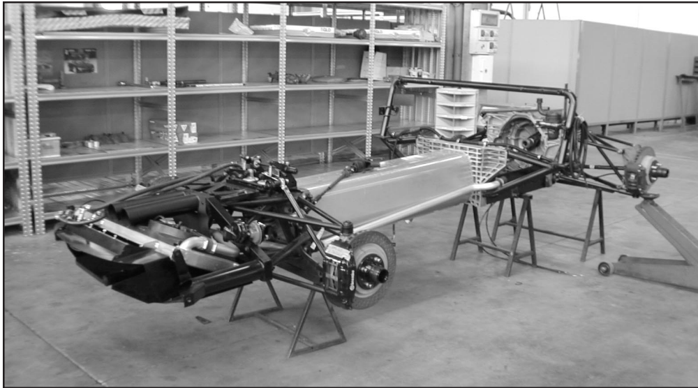
The central spine is the heart of the Guará's chassis. The front subframe holds the suspension and radiator, while two massive extrusions are joined by a cradle which supports the engine. The rear suspension attaches to the rear casting
