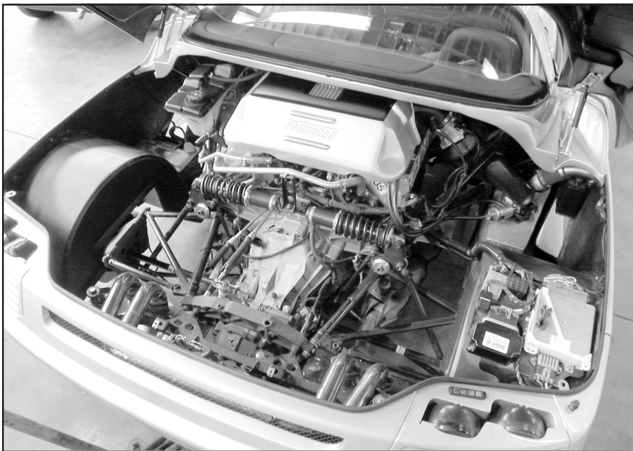
De Tomaso has done a masterful job of packaging. The highly advanced rear suspension attaches to castings, one between the engine and gearbox and the other attached to the rear of the gearbox
