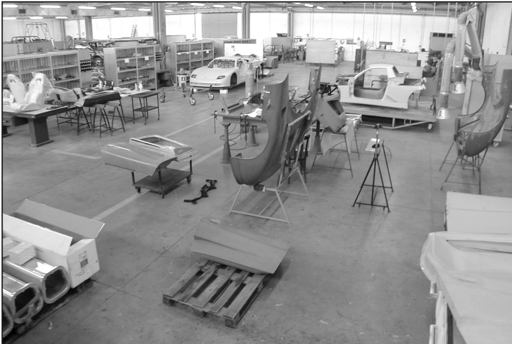
The Guará bodies take shape in this area, and final assembly takes place on the other side of the partition. The machine shop is at the rear of the building. Bare chassis lie on the pallet on the left
