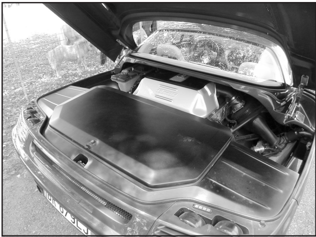
An insulated fiberglass box lies atop the gearbox to serve as a trunk, sized to hold two sets of golf clubs
