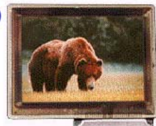
Sanyo Color AMOLED display - 852x222 pixels (prototype, 2.5" diag.) A 5-inch QVGA has also been shown
