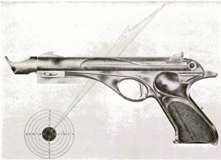
With racy appeal of Buck Rogers ray gun, artist's study of target model styling incorporated muzzle brake for rapid fire with front take-down bushing.
