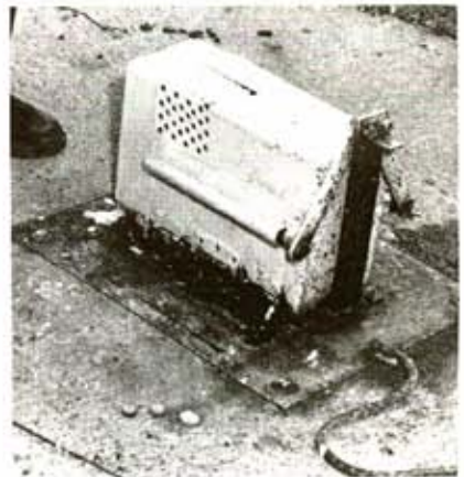
Traps are opened by pulling wires which release halves. Hose carries air blast that scares pigeon into flying away.
