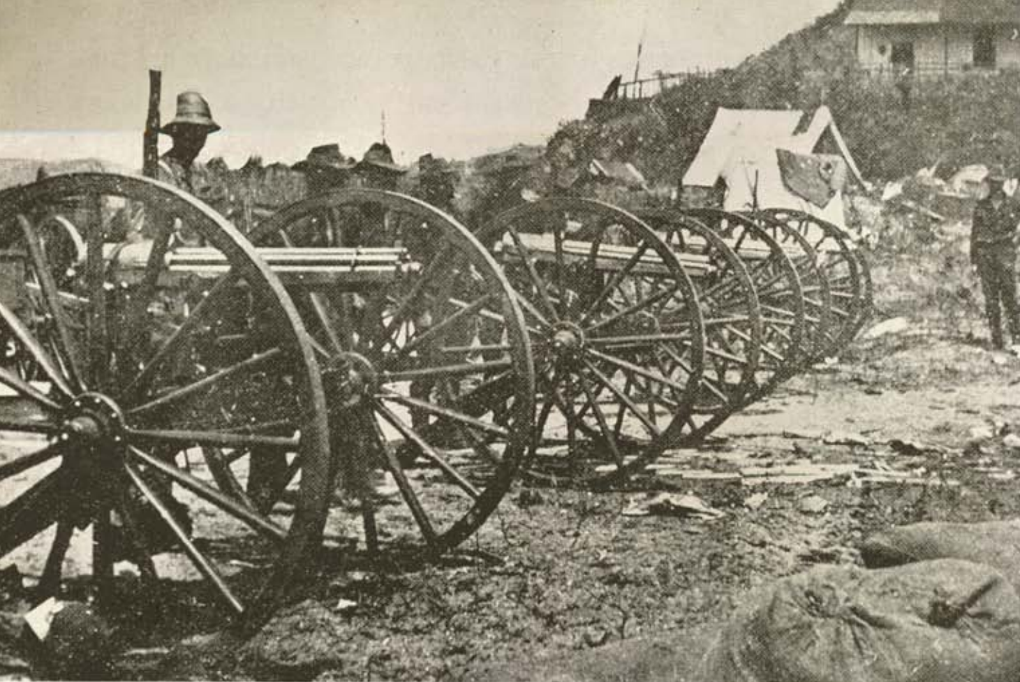
Model 1895 Gatling guns on steel field carriages with double-row Bruce feeds were unloaded at Daiquiri in Cuba ready to follow troops in combat under command of Lt. Parker who foresaw the value of machine gun tactics in combat.
