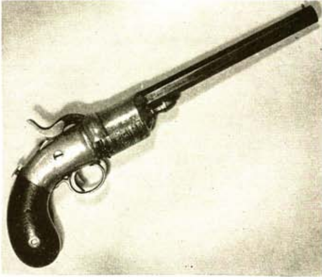
First pistol with name of "Whitney" was percussion revolver made in factory of Eli Whitney (right), whose son continued gun business until 1880's. Weapon coincidentally had cast metal frame for low-cost construction, like modern Whitney.
