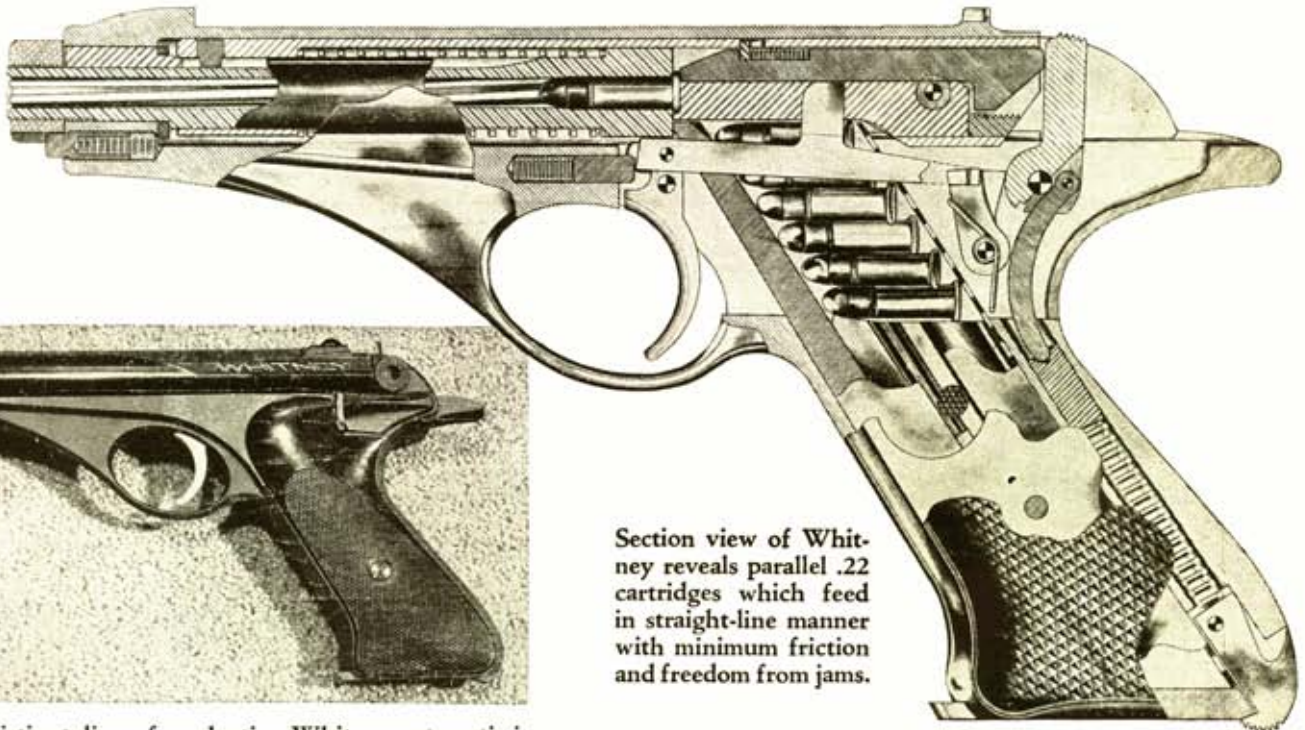
Futuristic styling of production Whitney automatic is enhanced by two-tone black anodizing finish. Thumb safety is fast, snaps off by thumb pressure upwards.
