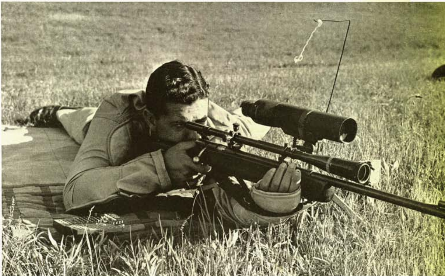
Because basic design of Mossberg .22 single shot was not adapted to reliable machine rest testing, accuracy firing was done with 20X scope fitted, and under careful range conditions to insure maximum, reliable performance of gun.
