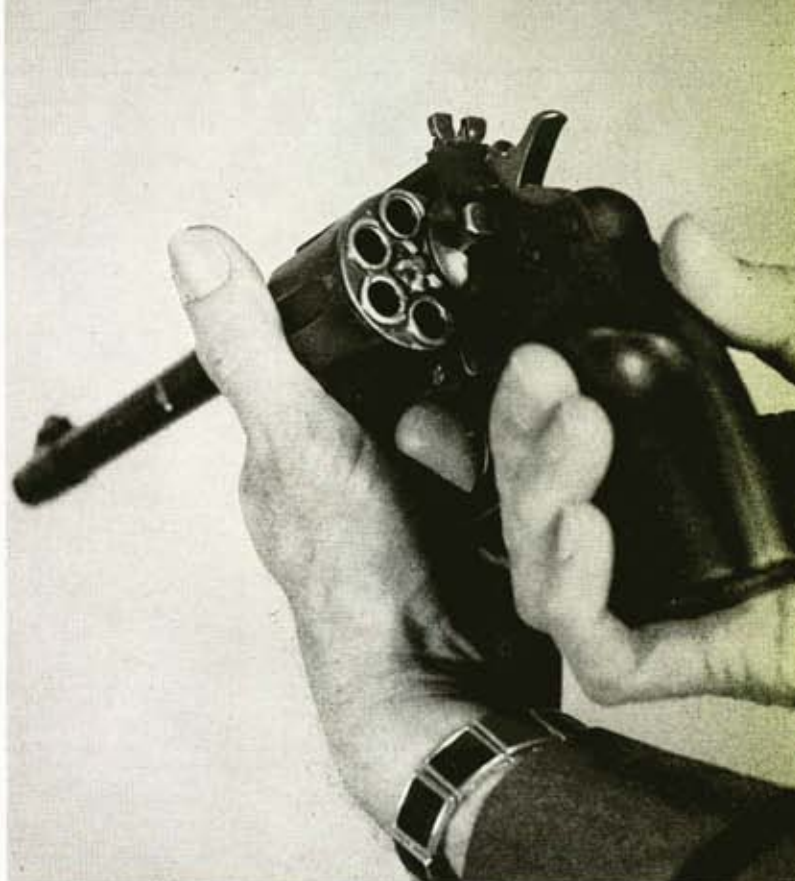
Chambers of .45 revolver were lined with tool steel bushings counterbored to recess case heads and then pressed in, which adapted gun to smaller cartridge.
