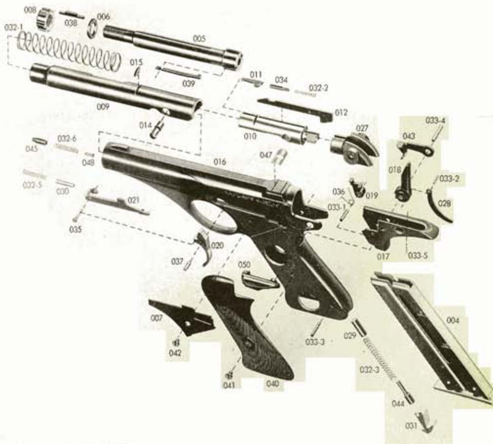
By assembling tubular and lathe-turned parts into precision die-cast frame unit, New Haven-built Whitney pistol is inexpensive yet sturdy and accurate.
