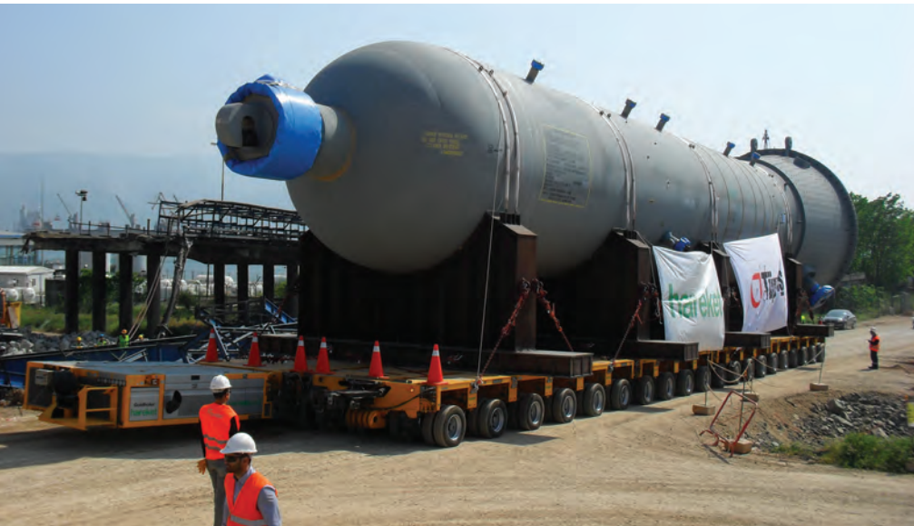
Above: A 918 tonne reactor is transported from Derince Port to Tupras refinery on 20 Goldhofer axle lines
