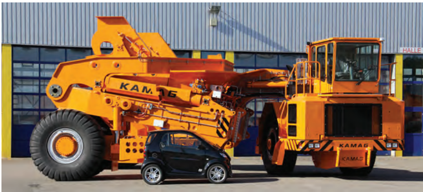
The 2802-130 type slag pot carrier has been designed to meet the needs of modern steel plants
