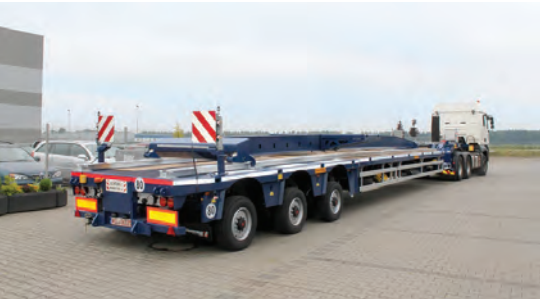
Faymonville released the Telemax trailer featuring a steering angle of up to 60° to help increase ground clearance
