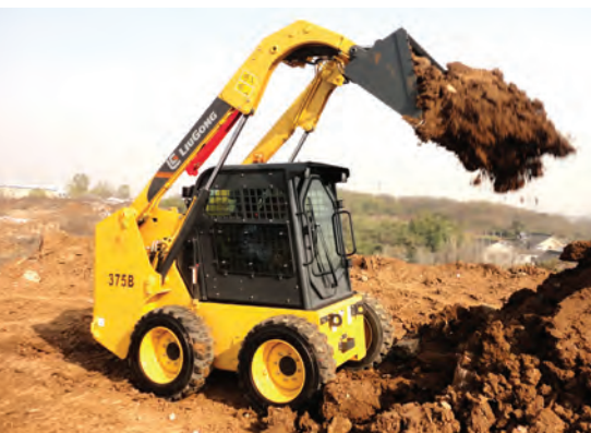
Liugong said it would present a new Tier 4 Final-compliant skid steer loader in the form of the 375B
