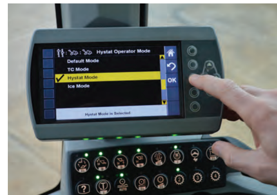
Cat is about to introduce hystat operator modes with three settings
