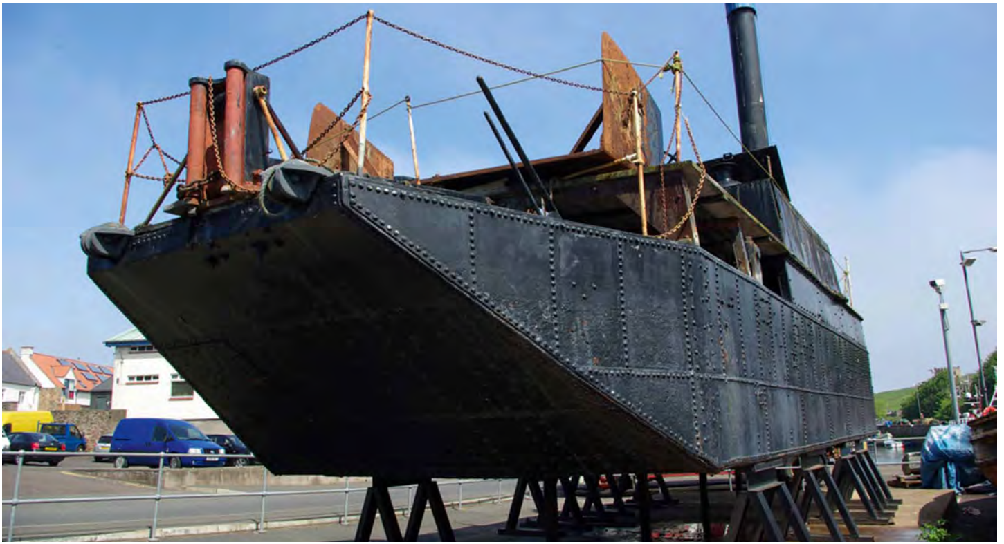
Fig 3. The chain-operated drag-boat Bertha was built in 1844 to act as a dredger for the inland port of Bridgwater. It is the oldest operational steam vessel in Britain, and now forms part of the International Sailing Craft Association collection and National Historic Fleet. She is on display at Eyemouth (Berwickshire).
