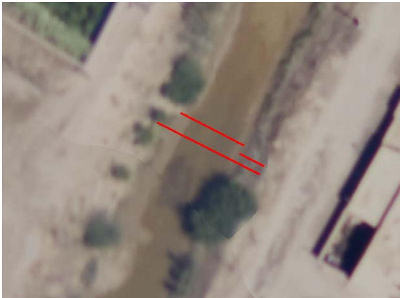
Figure 5. Representative Section of Sluice Channel: July 2010. Red lines are channel width, sediment width, and exposed sideslope width resp.
