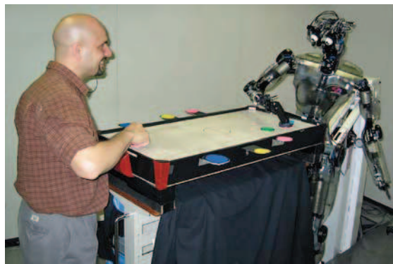
Fig. 56.22 The humanoid robot DB learns to play air hockey against a human opponent through observation and practice. ©JST, ATR; Robot developed by SARCOS
