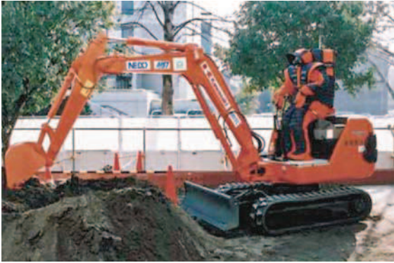
Fig. 56.1 The humanoid robot HRP-1S driving a backhoe (Courtesy of Kawasaki Heavy Industries, Tokyu Construction and AIST). The robot can be teleoperated by a human operator to control the backhoe remotely. The same robot could potentially interface with many different unmodified machines
