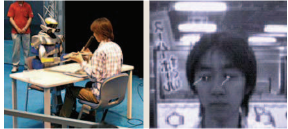
Fig. 56.43 HRP-2 recognizing face and gaze direction for communication via eye contact
