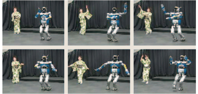
Fig. 56.3 The humanoid robot HRP-2 dancing with a human [56.22]. The human is a master of a traditional Japanese dance whose dancing was recorded by a motion-capture system, and transformed for use by the robot
