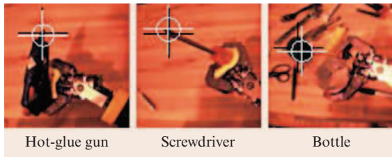
Fig. 56.18 Using visual motion, Domo detects ( white cross ) the tips of tool-like objects it is rigidly grasping with error ( white circle ) comparable to the error achieved with hand labels ( black cross )
