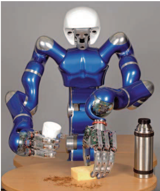
Fig. 56.16 The humanoid robot Justin has two seven-DOF torque-controlled arms ( DLR-Lightweight-Robot-III ), and two 12-DOF hands ( DLR-Hand-II ). Justin's body is larger than a human's
