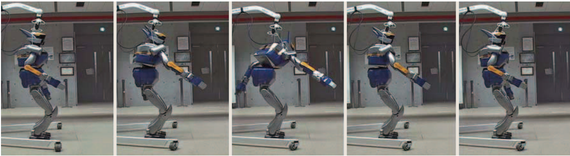
Fig. 56.33 Forward reaching motion with balance [56.75]
