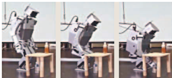
Fig. 56.32 The humanoid robot H7 executes a motion generated by the autobalancer [56.77]
