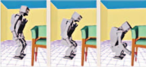
Fig. 56.29 An example whole-body motion generated by the RRT motion planning system [56.77]
