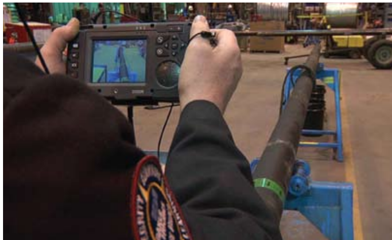
Video of the inspection of an electrical submersible pump (ESP) is sent from Centrilift repair workshop in Leduc, AB, Canada, to a remote facility.
